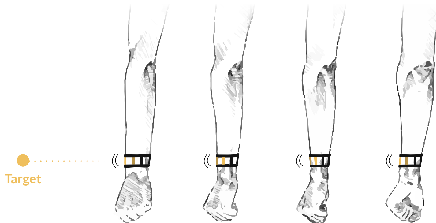
Figure 5: Showing different rotations of the wrist. Note how closest tactor to target is always vibrating.
